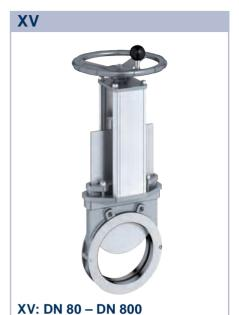
This compact knife gate valve is bi-directional and is designed for high differential pressures. Full passage and minimised clearance volumes result in a good flow characteristic. The flange ring system simplifies maintenance.
