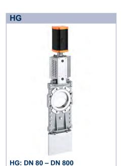
This knife gate valve is especially suitable for statically charged and highly corrosive media. Thanks to the through-hole in the gate, it has excellent flow characteristics and no media can accumulate in the passage.
