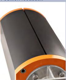
Integrated keyway in the housing for mounting limit switches in accordance with ISO 15552 for non-contact position detection when using magnetic pistons (optional).
